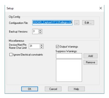
Select the Edit button and add a new Component Definition Property Component\_Height=HEIGHT. Save the allegro.cfg file and OK the setup dialog, then OK to create the netlist.
