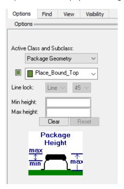
Set the Min (If required) and Max heights. If you only have one height only set the Max height. The min height is normally used if the component does not sit on the surface of the PCB directly. This gives users the option to place components underneath other components for example a DIP carrier has space below allowing surface mount components to be placed underneath the part. This is not a recommended design practice and can have
