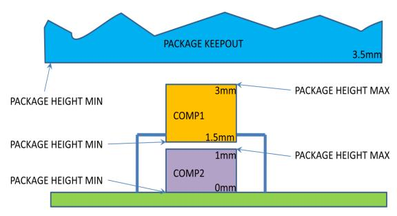
Note: If the Place\_Bound\_Shape (Top/Bottom) does not have a height defined then the shape will use the default component height specified from Setup – Design Parameters – Design Tab – Default Symbol Height.
