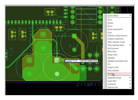
The 3D Viewer opens and displays the STEP model for this package symbol. The STEP model and pad stack (if set to be visible) are displayed in the 3D Viewer.
