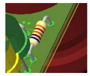
This is an example of a part that may be incorrectly defined in the library as the pins align, but the bodies do not.
