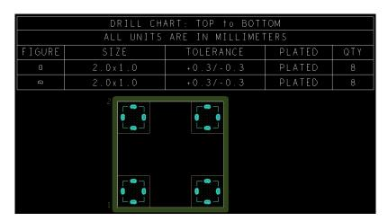
The NC Drill legend does reference the slots (as shown below) but the NC Drill does not reference the slots. You will see a WARNING in the NC Drill file that the slots cannot be drilled and must be routed:-
