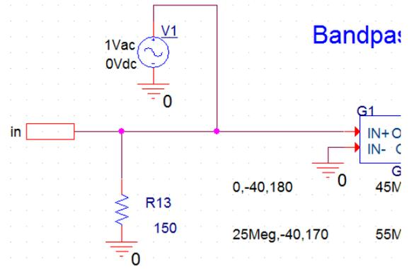
We are now ready to run the PSpice simulation. We will start by creating a new simulation profile, PSpice – New Simulation Profile, specify a name AC and click on Create.
