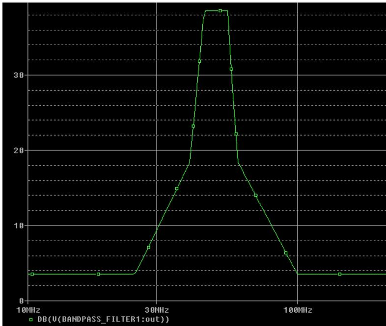
If the desired output does not meet the requirements you can adjust the resistance values and re-run the simulation. In this instance we will change the resistance value of R14 from 150 to 250 ohms resulting in:-
