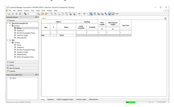
There are more columns in the Electrical>Net>Routing>Wiring Worksheet because the Net Worksheets will show the Actual values for the routing and Margins between the routed Nets and the Constraints set for them.
