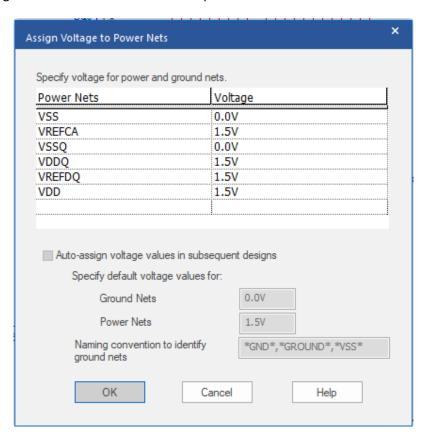
Assign appropriate voltages to the Voltage Nets. (Use the Auto Assign settings to automatically assign Voltages to Power Nets in other designs opened and Constraint Manager enabled in the same Capture session)
