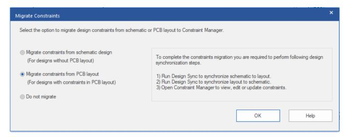
Left-click>OK and the steps from the form MUST be then performed, in order, to complete the Constraint Manager enabled flow migration:
