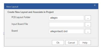
Leave the defaults and click OK. You will notice the board file is created and shown in the Project window under the Layout section. Now choose PCB>Design Sync again and change the arrow from Schematic to Layout to Schematic (Left click the arrow) the click on Sync.
