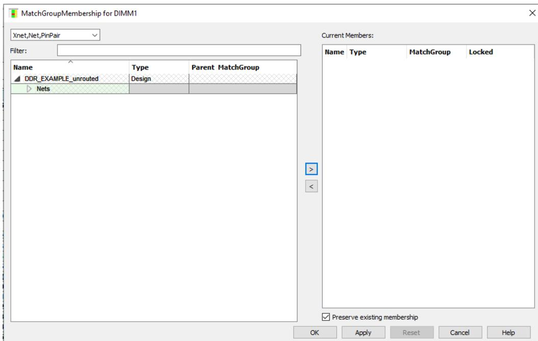
To generate the PinPairs quickly open the Min/Max Propagation Delay worksheet and specify a value for Min length for the Address and Bytelane classes (1mm will do) and OrCAD Professional automatically generates all the relevant pin pairs.
