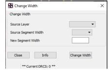
Specify the Source layer, source segment width and new segment then click on Change Width. This changes all clines on the source layer to the new width. As with the other methods if this is new value is outside of the min/max values in Constraint Manager you may invoke a DRC Marker. Adjust the values in Constraint Manager to suit.
