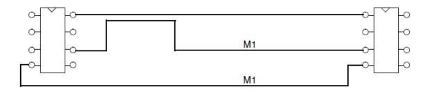
You can create Match Groups manually by adding properties directly to Xnets, or by using Constraint Manager to explicitly define pin pairs in an Electrical CSet. Regardless of the method that you choose, Match Groups are resolved down to specific pin pairs and are further defined by the following attributes: Scope, Delta, Tolerance and Target.
