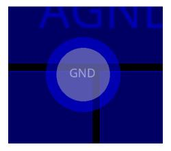
The final option does not use a pin or pins to create the net short but simply a small area of copper. You can add a static shape copper area to create the short between two other shapes on a specific layer of the PCB. The steps are described below.
