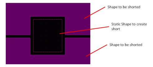
You now need to add properties to the static shape to create the required effect. To do this use Edit > Properties (Allegro) or Edit > Object Properties (OrCAD) then making sure you have Shapes selected in the Find Filter, select the static shape with a left click, you will see the following property edit window:-
