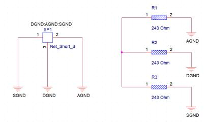
On each pin on the net short (SP1) you will need to Edit Property (Double click the pin) and add the net names that you wish to short separated by a colon. In this example the nets are DGND:AGND:SGND. It is recommended that for each pin the primary net is first (i.e. pin 1 the NET\_SHORT would equal SGND:AGND:DGND. You also need to ensure that you also have a PCB footprint defined for the netshort part.
