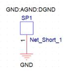
For the PCB only a single PAD is used and in the picture below shows the pad crossing the boundary of the three nets GND, GND\_EARTH and AGND. This example also means that there are no extra DRC's that need to be waived or extra properties required but the main disadvantage of this is that there is only one connection for this pin (GND). This means that you will have no feedback whether you make the short to AGND and GND\_EARTH.
