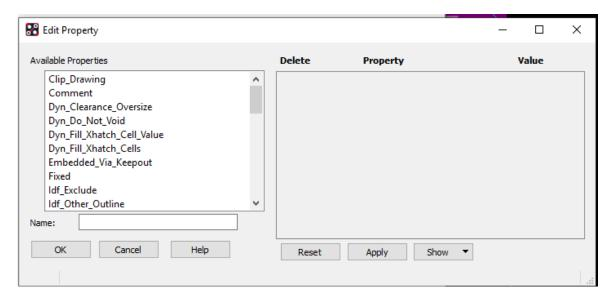
Locate the property name Dyn\_Do\_Not\_Void and click on Apply. This property is added to stop the dynamic shapes from voiding the static one. Locate the property Net\_Short and left click to select the property, you now need to add the two net names you wish to short together in the format netname1:netname2, for this example it's AGND:DGND.
