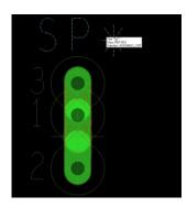
Open the board file and import the netlist from Capture. Place your components. You will notice in the next screenshot that the net short SP1 is placed and there are no DRC errors.
