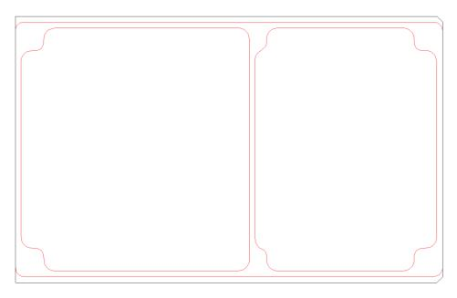
To create a soldermask clearance area we need to use the compose shape command. Shape > Compose Shape (In Allegro) or Shape > Create Shape From Lines (in OrCAD), in the Options menu select Board Geometry / Soldermask\_Top as the Active class / subclass.
