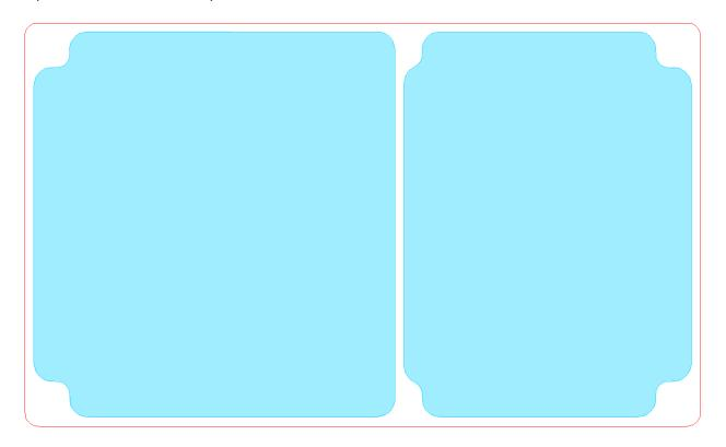
Finally draw a box around all items (The two inner shapes and the surrounding profile. PCB Editor will use the outer outline as the master shape and will subtract the two inner shapes, leaving you with the resulting figure.
