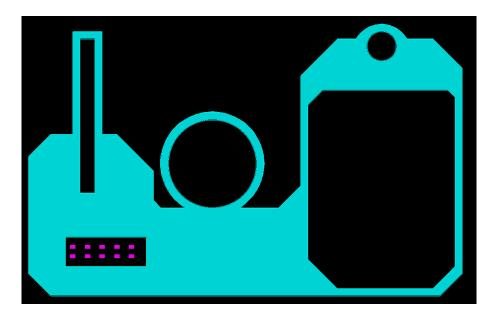
If you use the soldermask to soldermask DRC checks found under Setup > Constraints > Modes (in Allegro) or Setup > Constraint Modes (in OrCAD) then you will need to clear areas where component padstacks are using the Shape > Manual Void (in Allegro) or Shape > Manual Isolation/Cavity (in OrCAD) functions as described earlier. An example of this is shown above where the purple pads represent five 1206 resistors.
