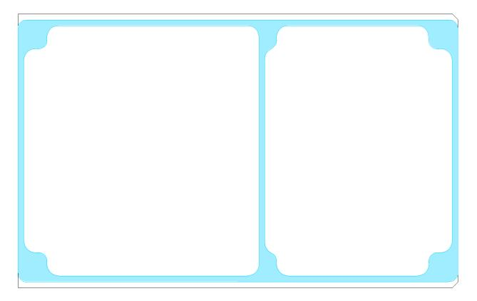
You can use the Edit > Z-copy command (Allegro) or Shape > Z-Copy (OrCAD) to copy this to the Soldermask\_Bottom layer or Etch layers to match the metalwork profile layers. If you use Z-copy to create etch shapes, ensure that you generate dynamic shapes so that any voids required are generated.
