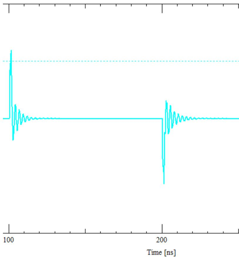
Few systems would be analysed for such a low frequency signal but just look at the excessive ringing in the victim, almost 30% of the signal voltage. Also note that additional transitions from other adjacent connections would only compound the misery!
