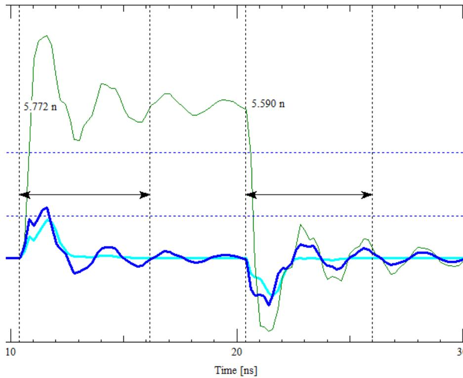
Note that the “un-terminated” driver gets enough energy at the receiver to cross the  $V_{il}$  threshold! Just as a reminder of what could possibly go wrong, change the custom stimulus to use a 10MHz frequency and re-run the simulation.
