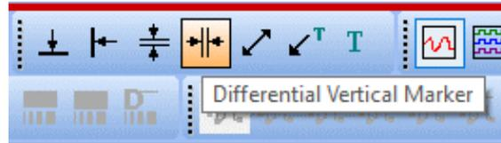
Place the first Differential Vertical marker between the start and end of the rising transition and a second between the start and end of the falling edge. The marker will be added to the waveform, click on one of the vertical dotted lines and hover to get the "double arrow" cursor, then drag the vertical dotted lines to the required locations.
