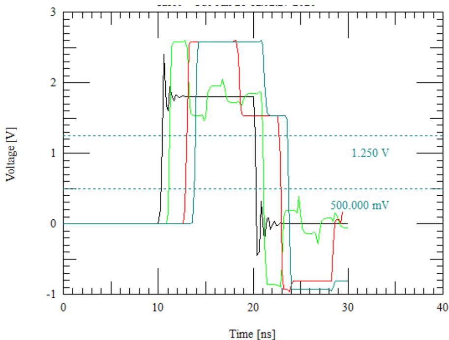
The green trace above, for the 5000 Mils case, shows the signal being repeatedly “bounced” from end to end of the trace. This will be the setting used for the next section to investigate the effects of changing the impedance of the microstrip on the reflections.
