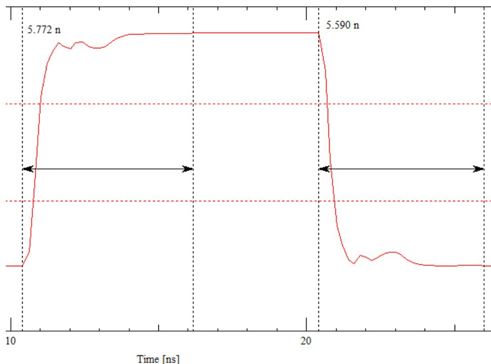
Now hide the Receiver waveform and display only the Victim waveform. Leave SigWave open, go back to SigXplorer and remove the termination for the driver connection (set the termination value to 0) and re-run the simulation. Set the waveform in SigWave to display the Victim in each case. Use the Line Color and Line Width to tweak the displayed waveforms to improve visibility.
