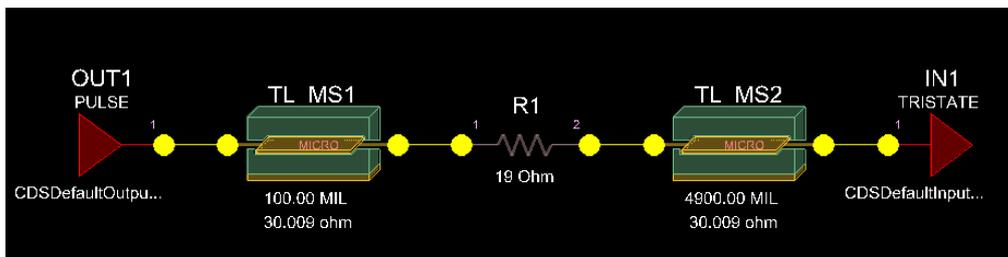
Change the resistor value to 19 Ohms and set the parameters of the microstrip sections to be d1Thickness=3.05 Mils, traceWidth=12 Mils, length for TL\_MS1 to 100 Mils and TL\_MS2 to 4900 Mils. This will clear the Impedance display in the canvas, to restore this, select the TL\_MS parts in turn and right-click>View Trace Parameters to update the Impedance values, they should both be 30 Ohms. The output impedance of the driver is about 11
