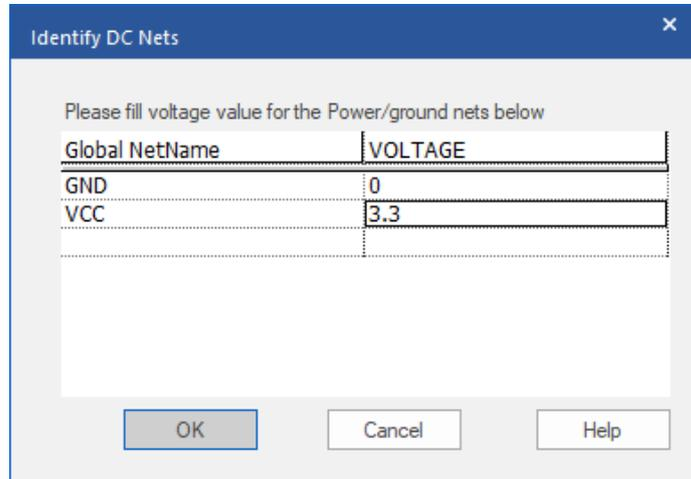
Once the SI Models have been assigned and the DC voltages defined, the topology can be exported to SigXplorer for analysis. With an OrCAD PCB SI, or higher, license you can select the net in the schematic page and right-click>SI Analysis>Explore Signal (SigXplorer). For an OrCAD PCB Designer Professional license, you would need to select the net in the schematic page and right-click>SI Analysis>Export Topology which writes a netname.top file that can be opened from SigXplorer.
