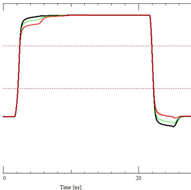
The Black trace is the 17 Ohms case and the Red trace is the 22 Ohms case. See that the smaller terminator value has a “clean” rising edge but has some amount of negative overshoot on the falling edge, whereas the larger value has removed the negative overshoot, the rising edge is now starting to show some undershoot. Like many things in engineering, the final solution is likely to be a compromise based upon the availability of “real” components values for the terminating resistor.
