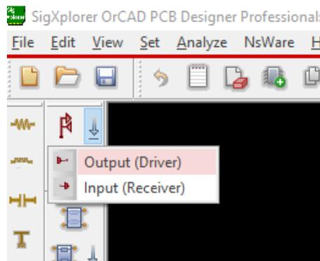
Use the Transmission Line icon on the left to place a piece of Microstrip and then add an Input (Receiver)
