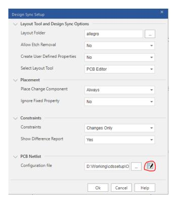
Add the following line to the section for [ComponentInstanceProps] DESIGN\_NOTE=YES.
